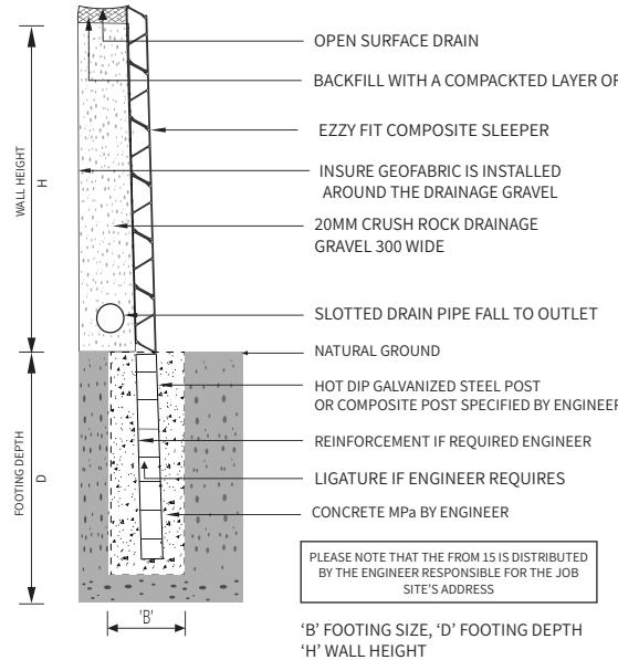
Wall heights exceeding 1 mtr must be designed by the responsible engineer overseeing the project. The diagram provided below is intended for reference purposes only.
